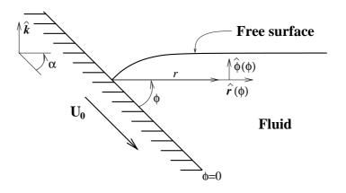
Figure 4: A plate is inserted into a semi-infinite domain of fluid at a constant velocity  $\mathbf{U}_0$ . The angle between the plate and the free surface at  $r \to \infty$  is  $\alpha$ .
