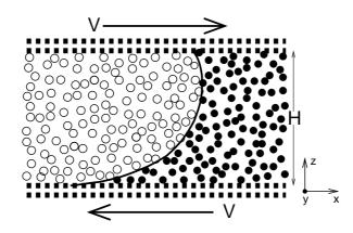
Figure 10: Schematic of the immiscible Couette flow. Two immiscible fluids (empty and solid circles) are confined between two solid walls (solid squares) that are parallel to the xy plane and separated by a distance H. The Couette flow is generated by moving the top and bottom walls at a speed V along  $\pm x$ , respectively.
