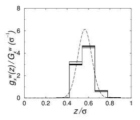
Figure 13: Subdividing the BL into thin sections, we plot the reduced tangential wall force density as a function of distance z away from the boundary. The solid lines are averaged  $g_x^w(z)$  in thin sections at different x, normalized by the corresponding total wall force per unit area. The dashed line is a smooth Gaussian fit. It is seen that  $g_x^w(z)$  is a function sharply peaked at  $z \approx z_0/2$ . Note that  $\int_0^{z_0} dz [g_x^w(x,z)/G_x^w(x)] = 1$ .
