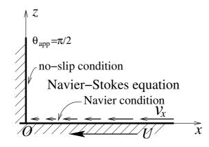
Figure 9: Two-dimensional corner flow caused by one rigid plane sliding over another, with constant inclination  $\theta_{app} = 90^{\circ}$ . In the reference frame of the vertical plane, the horizontal plane is moving to the left with constant speed U.
