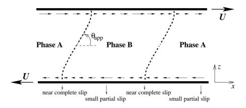
Figure 5: The xz projection of the simulated system. Thick solid lines represent solid walls and dashed lines represent fluid-fluid interfaces. The arrows indicate fluid velocity close to the solid walls, from which the variation of the amount of slip is clearly seen.
