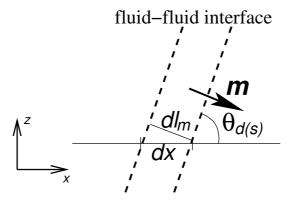
Figure 29: Schematic illustration for the origin of the tangential Young stress  $\sigma_{zx}^{Y(0)}$  as an off-diagonal component of the microscopic stress tensor.
