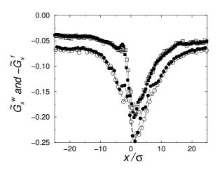
Figure 27: Hydrodynamic force balance for the lower BL. The circles represent the symmetric case  $(V = 0.25\sqrt{\epsilon/m} \text{ and } H = 13.6\sigma)$ ; the squares represent the asymmetric case  $(V = 0.2\sqrt{\epsilon/m} \text{ and } H = 13.6\sigma)$ . The empty symbols denote  $\tilde{G}_x^w$ ; the solid symbols denote  $-\tilde{G}_x^f$ . It is seen that  $\tilde{G}_x^w(x) = -\tilde{G}_x^f(x)$ .
