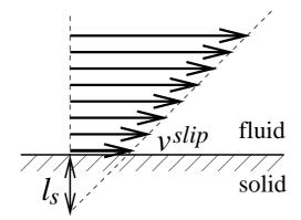
Figure 1: Slip length introduced in the Navier boundary condition, defined as the distance from the fluid-solid interface to where the linearly extrapolated tangential velocity vanishes.
