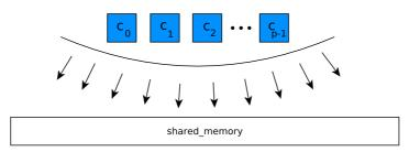
Figure 3: In the PRAM model each one of the cores has a complete view of the global memory.
