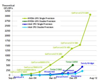
Figure 2: Comparison of CPU and GPU single precision floating point performance through the years. Image taken from Nvidia's *CUDA C programming guide* [93].
