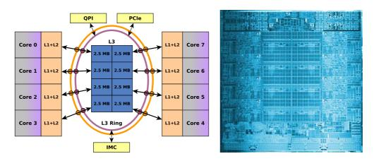
Figure 9: On the left, an Intel Xeon E5 2600 (2012) chip schematic, inspired from [28]. On the right, the processor die [57].
