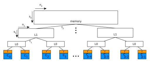
Figure 4: The uniform parallel memory hierarchy tree.
