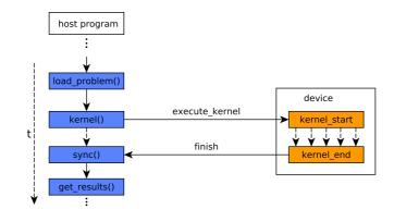
Figure 15: The GPU's main function, named kernel, is invoked from the CPU host code.
