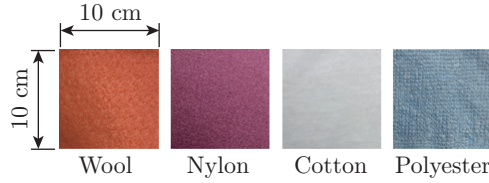
Fig. 1: Wool, Nylon, Cotton and Polyester fabric samples evaluated in the study. Each sample was 10 cm \times 10 cm in size. Insulation characteristics and IR radiation attenuation properties were evaluated for 1, 2, 4, and 6 layer combinations
