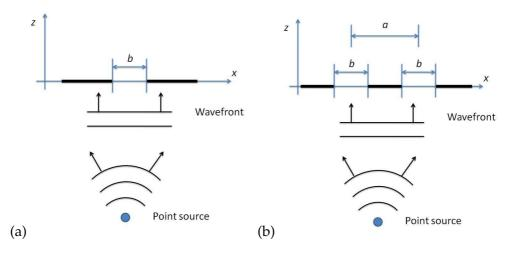
Figure 1: Setup for (a) single slit diffraction and (b) double dlit diffraction.
