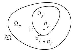
Figure 1: Sketch of a free flow region  $\Omega_f$ , a porous media region  $\Omega_p$ , and the interface  $\Gamma$ , the normal direction  $n_f$  and tangential direction  $\tau_j$ , as well as boundary  $\partial\Omega$ .
