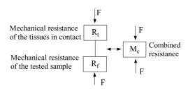
Figure 2 Equivalent mechanical sensing system
