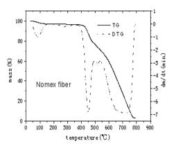
Figure 2 The TG and DTG curves of Nomex fiber.
