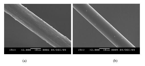
Figure 1 Longitudinal micrographs of Nomex and Kevlar 49 fiber. a Nomex fiber. b Kevlar 49 fiber.
