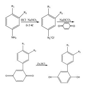
Scheme 1. Synthesis of bisphenol monomers. (4-fluoro)phenylhydroquinone: R<sub>1</sub>:F, R<sub>2</sub>:H; (3,4-bifluoro) phenylhydroquinone: R<sub>1</sub>:F, R<sub>2</sub>:F
