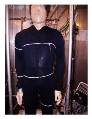
Figure 1 The thermal manikin 'Tore' in the climatic chamber.
