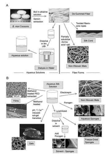
Figure 1. (A) Silkfibroin is purified from sericins via boiling in an alkaline solution. (B) Processing of silk morphologies from aqueous silk fibroin solution [17].
