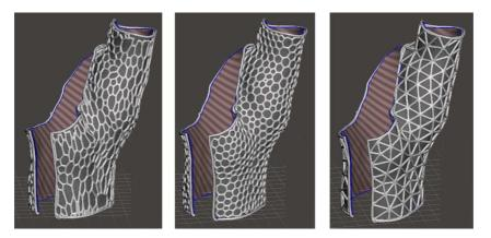
Figure 1: Different structures by using Autodesk Meshmixer free software. Reprinted from Fernandez-Vicente et al. [13] with permission from Rapid Prototyping Journal.
