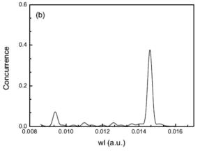
Figure 2: The mean values of the concurrence over long time T for initial state |0,2) as a function of laser frequency
