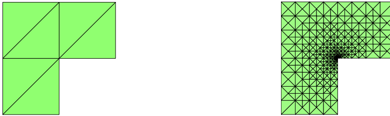
(a) Initial grid: isosceles triangles. (b) Adaptive grid obtained by newest vertex bisections.
