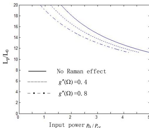
Figure 2: The relationship between the effective polarization beat length and the input power when the parallel Raman gains are 0, 0.4, 0.8 respectively.
