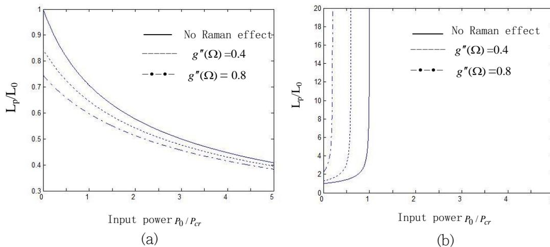
Figure 1: (a) The relationship between the effective polarization beat length and the input power when the parallel Raman gains are 0, 0.4, 0.8 respectively. (b) The relationship between the effective polarization beat length and the input power when the parallel Raman gains are 0, 0.4, 0.8 respectively.
