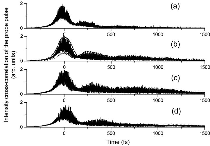
Figure 3: Experimental results. Temporal behaviour of the  $\sigma$  pulse for an atomic system driven by a strong field which energy is (a) 80 (b) 150 (c) 200 (d) 300  $\mu\text{J}$ . See text for experimental parameters. The phase fluctuation is responsible for the rapid variations.
