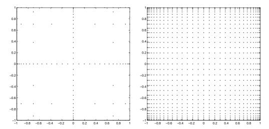
Figure 1: Two-dimensional (N=2) nodes based on the extrema of Chebyshev polynomials. Left: Sparse grid from Smolyak algorithm. Total number of points is 145. Right: Tensor product grid constructed from the same one-dimensional nodes. Total number of nodes is 1,089.
