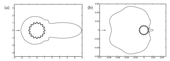
Figure 7: Acoustic scattering over cylinder with rough surface. The arrow indicates the direction of the incident plane wave. (a) The mean solution of RCS. The thick line is the mean boundary of the gear-shaped obstable; (b) Standard deviation of the RCS profile. Here the thick line is only a reference of the location of the obstable because of the scale difference.
