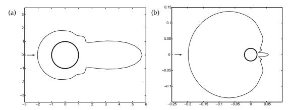
Figure 5: Acoustic scattering over cylinder with rough surface. The arrow indicates the direction of the incident plane wave. (a) The mean solution of RCS. The thick circle is the mean boundary of the scatterer; (b) Standard deviation of the RCS profile. Here the thick circle is only a reference of the location of the cylinder because of the scale difference.
