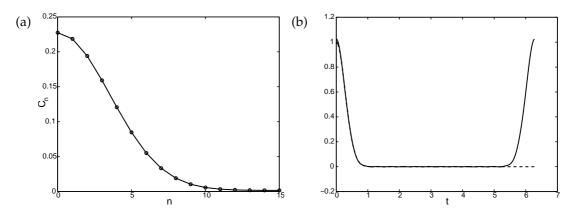
Figure 3: Construction of a  $2\pi$ -periodic covariance function  $C_f$ . (a) Decay of Fourier cosine coefficients  $C_n, n=0,1,\cdots$ ; (b) Reconstructed periodic covariance function (solid line) by extending the regular Gaussian covariance function (dashed line)  $C_G(t)=\exp(t^2/b^2)$  with correlation length b=0.4.
