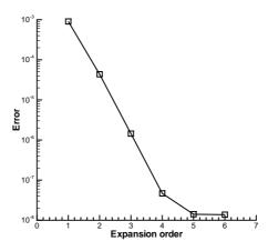
Figure 2: Mean square errors of model case with increasing order of gPC expansions.
