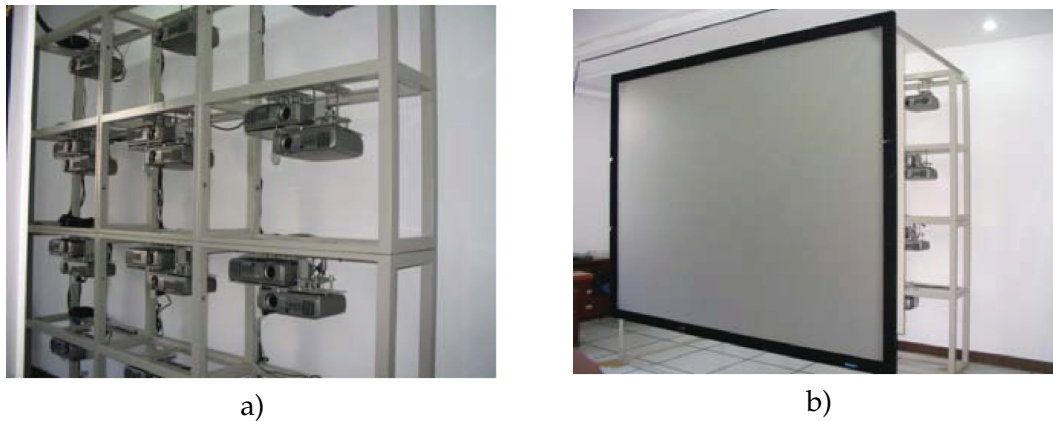
Figure 5: A typical stereo display wall system supported by a PC cluster: a) A matrix of projectors; and b) A screen and projectors.
