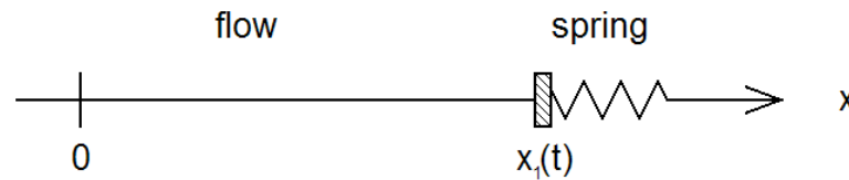
Figure 1: A one-dimensional flow problem interacting with a spring.
