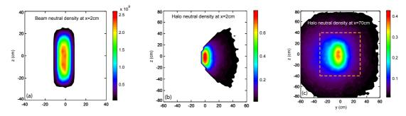
Figure 11: Vertical (y,z) planes of (a) injected neutral density near the plasma edge, (b) halo neutral density near the plasma edge, and (c) halo neutral density in the plasma interior.
