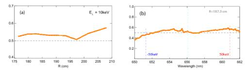
Figure 13: (a) Ratio of the blue-shifted FIDA radiance for simulations without halo neutrals and with halo neutrals vs. major radius. The spectra are integrated over wavelengths above  $E_{\lambda}=10 \mathrm{keV}$ . (b) Ratio of the FIDA spectral radiance for simulations without halo neutrals and with halo neutrals for the FIDA channel at  $R=187.5 \mathrm{cm}$ . Two values of  $E_{\lambda}$  are indicated.
