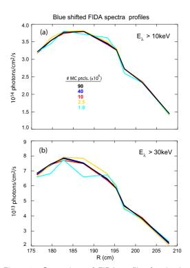
Figure 9: Comparison of FIDA profiles for simulations with  $10^6$  to  $9\times 10^7$  Monte Carlo particles. The spectra are integrated over Doppler shifts larger than (a)  $E_\lambda \geq 10 {\rm keV}$  and (b)  $E_\lambda \geq 30 {\rm keV}$ .
