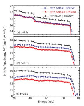
Figure 6: NPA energy spectra for a sightline with  $R_{tan} = 70 \mathrm{cm}$  from the TRANSP and FIDASIM simulations with and without halos at three different times in NSTX discharge #122631. The density increased from approximately  $2 \times 10^{13} \mathrm{cm}^{-3}$  to  $5 \times 10^{13} \mathrm{cm}^{-3}$  between 0.1 and 0.5s.
