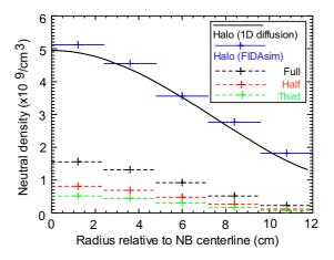
Figure 7: Comparison of halo neutral densities calculated from the 1-D diffusion model (Eq. (3.3)) and the FIDASIM halo diffusion subroutine for plasma profiles with  $n_i = n_e = 1.1 \times 10^{14} \text{ cm}^{-3}$ ,  $T_e = 2.5 \text{keV}$  and  $T_i = 1.25 \text{keV}$ . The three dashed steps represent the densities of the full, half, and third energy components of injected neutrals used in both codes.
