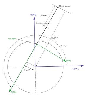
Figure 2: Plan view of NSTX. Geometrical neutral beam and detector input to the code is in (u,v,z) coordinates. Neutral beam parameters (upper case labels) follow the TRANSP conventions. The code transforms quantities into (x,y,z) coordinates along the selected beam.
