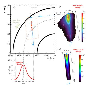
Figure 10: (a) Midplane (z=0) cross section of a quadrant of the DIII-D tokamak, showing the intersection of the vertical FIDA sightlines (triangles) and the (x,y) coordinate system associated with the active neutral beam. (b) Midplane halo neutral density. The distribution is asymmetrical due to the plasma flow. (c) Beam-ion density. (d) Injected neutral density.
