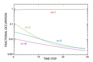
Figure 3: Solution of Eq. (2.3) immediately following neutralization of the fast ion for a typical case (density of  $4\times10^{13} {\rm cm}^{-3}$ , temperature of 4keV). The total time represented by the abscissa is 11.1ns; the fast neutral travels 3cm during this time. The evolution of the n=3 state determines the intensity of FIDA light.
