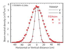
Figure 4: Comparison of injected neutral density profile along the y and z axes from the FIDASIM code (symbols) and from TRANSP (lines) at the beam tangency point ( $R\!=\!70\mathrm{cm}$ ) for NSTX Source A.
