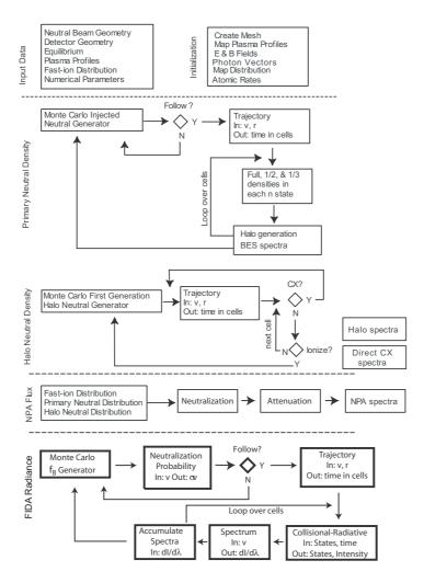
Figure 1: Flow diagram for the FIDASIM code.
