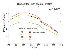
Figure 12: Dependence of the calculated FIDA radiance on the volume of the simulation. The spectra are integrated over wavelengths above  $E_\lambda = 10 {\rm keV}$ .
