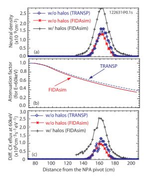
Figure 5: Comparison between the FIDASIM and TRANSP simulations in NSTX discharge #122631 at  $t\!=\!0.1s$ . (a) Neutral density, (b) attenuation factor for 60 keV neutrals and (c) differential charge-exchange flux along the NPA sightline.
