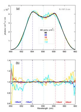
Figure 8: (a) Comparison of FIDA spectra from simulations with  $10^6$  to  $9\times 10^7$  Monte Carlo particles. (The reduction in FIDA light for small Doppler shifts is an artifact caused by truncating the fast-ion distribution function at  $E_{\rm min}=10{\rm keV.}$ ) (b) FIDA spectra normalized to the spectrum computed with 90 million particles. The dashed vertical lines relate Doppler shifts to equivalent energies along the line-of-sight  $E_{\lambda}.$
