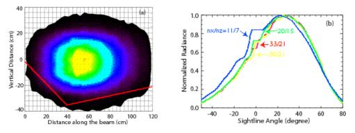
Figure 14: (a) FIDA emissivity in an (x,z) plane, with the standard  $(33\times21)$  grid boundaries overlaid. The red lines illustrate the range of sightline angles graphed in the lower figure. (b) Calculated radiance vs. sightline angle for different choices of grid size in the (x,z) plane. The flat portions of the curves are caused by pixelation.
