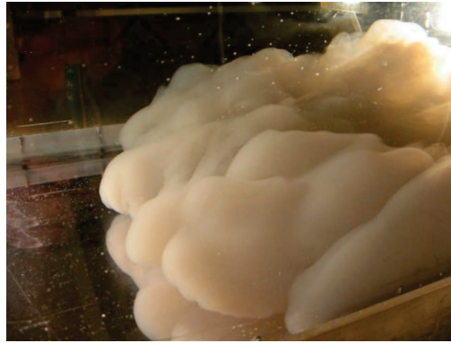
Figure 2: Tank experiment of a sand-laden multicomponent flow. The image is from [4].
