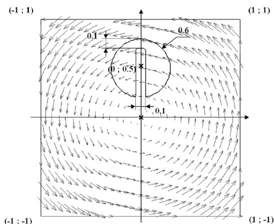
Figure 11: Simulation settings for the advection of a slotted disk. Velocity field:  $u_x = -2\pi \cdot y$ ;  $u_y = 2\pi \cdot x$ .
