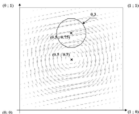
Figure 12: Simulation settings for the disk in a deformation field. Velocity field for  $t \in [0, 3](s)$ :  $u_x = -\partial\psi/\partial y$ ;  $u_y = \partial\psi/\partial x$ , with:  $\psi = \pi^{-1} \sin^2(\pi x) \sin^2(\pi y)$ .
