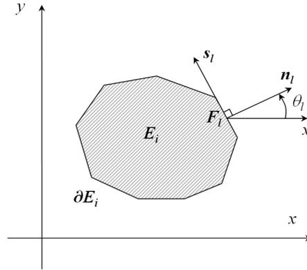
Figure 9: Rotated Cartesian frame in 2D:  $(n_l, s_l)$  — the first axis  $n_l$  is orthogonal to the arbitrary boundary  $\partial E_i$  of the control volume  $E_i$ .
