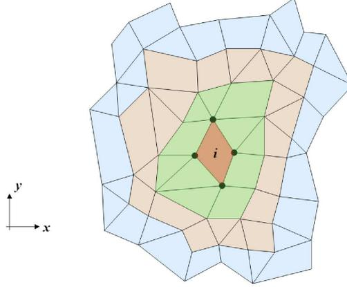
Figure 2: Layers of cells added to the dynamic list at each iteration: in indigo, the cells added at the 1<sup>st</sup> iteration; in blue, the cells added at the 2<sup>nd</sup> iteration — in 2D.
