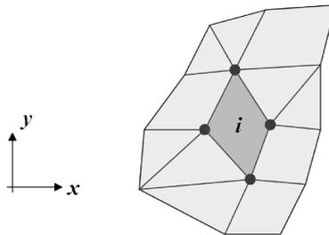
Figure 1: Schematic of the point-neighbours (light grey) of a targeted cell (dark grey) — in 2D.
