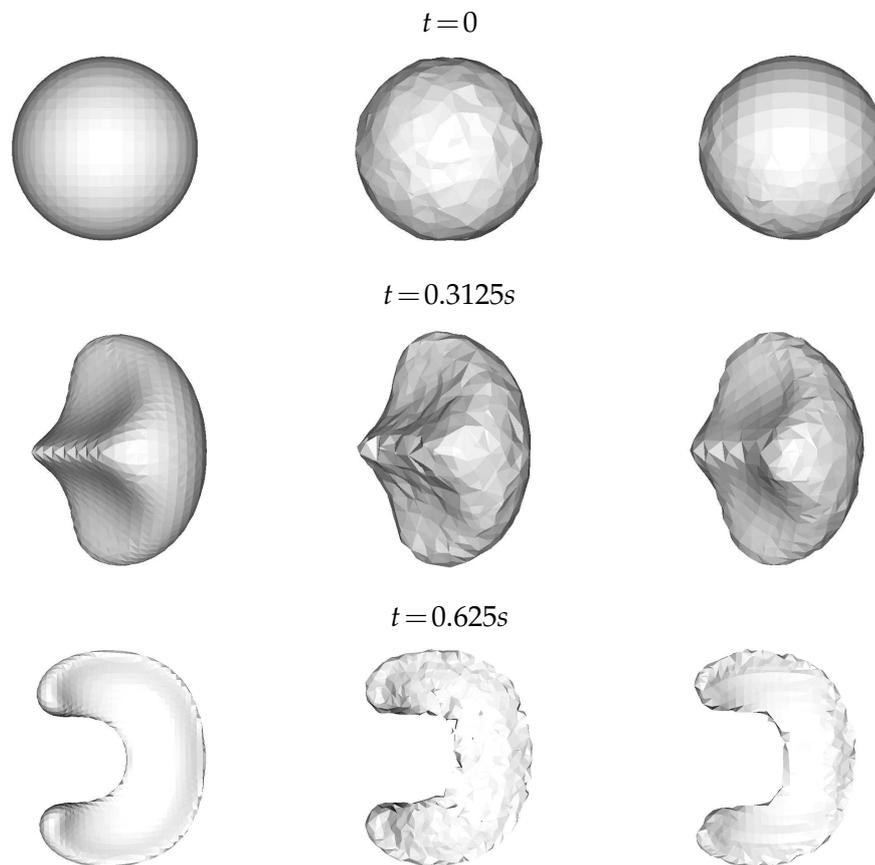
Figure 14: Zero level set for the sphere in a deformation field — Time  $t=0s, 0.3125s, 0.625s$ . Left: Cartesian mesh; Middle: Tetrahedral mesh; Right: Hybrid mesh.
