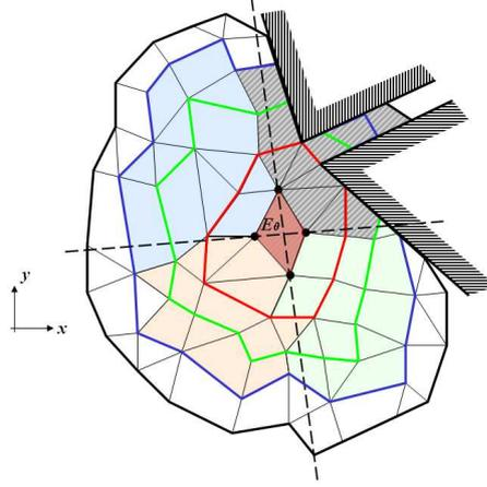
Figure 8: Thirteen-cells sectoral stencils of  $E_0$  coloured by sector: the colored thick lines indicate the progression of the search; discarded stencil hatched in grey; domain boundaries hatched in black-as produced by the fast search procedure in 2D.
