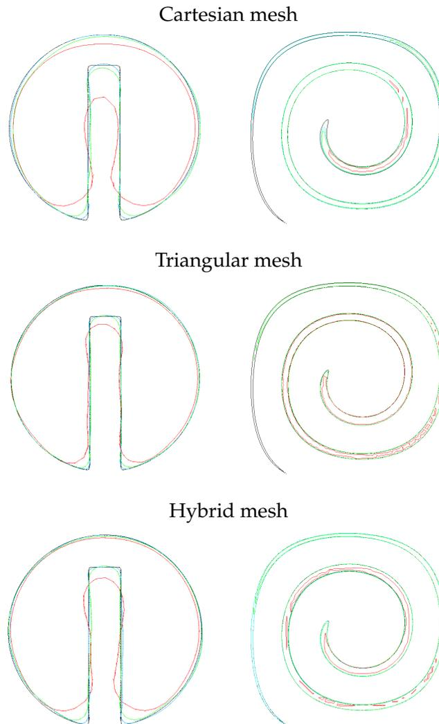
Figure 13: Zero level set for the translation of a slotted disk and the disk in a deformation field — in black: the reference; in red: solution for  $L/64$ ; in green: solution for  $L/128$ ; in blue: solution for  $L/256$ . Left column: translation of slotted disk; Right column: disk in a deformation field.
