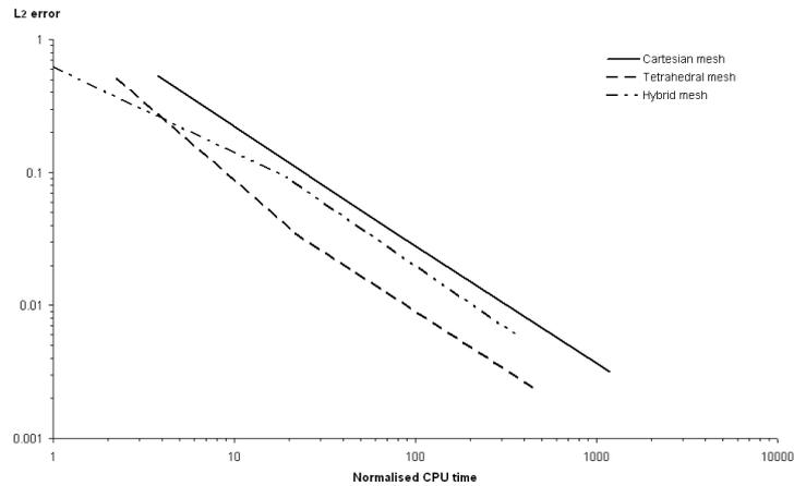
Figure 15:  $L^2$  error vs. normalised CPU time for the WENO3 applied to the linear equation.
