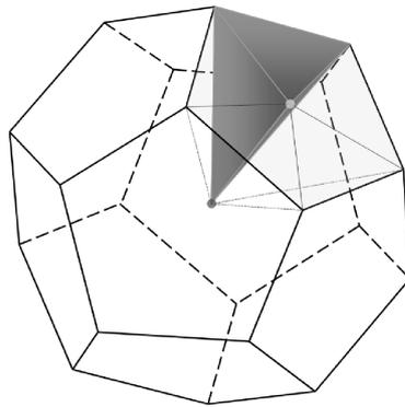
Figure 4: Tetrahedralisation of a convex polyhedron — in solid grey: a sub-element; thin lines: construction lines for the sub-elements; dark grey point: cell centre; shaded face: face decomposed; light grey point: centre of the face considered.
