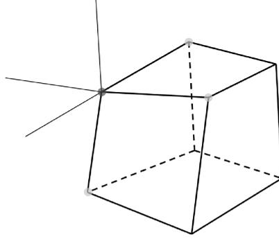
Figure 3: Schematic of the edge-neighbours (light grey vertices) of a given point (dark grey vertex) in a given cell (thick lines) — for a hexahedral cell.
