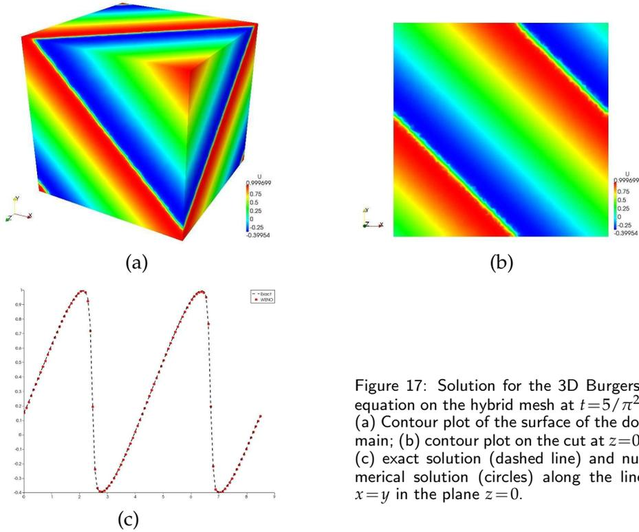
Figure 17: Solution for the 3D Burgers' equation on the hybrid mesh at  $t=5/\pi^2$ . (a) Contour plot of the surface of the domain; (b) contour plot on the cut at  $z=0$ ; (c) exact solution (dashed line) and numerical solution (circles) along the line  $x=y$  in the plane  $z=0$ .
