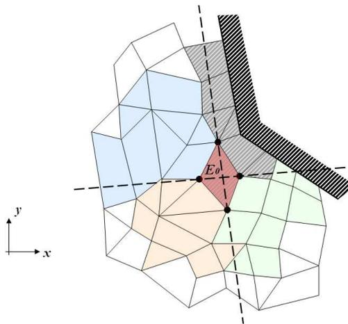
Figure 6: Ten-cells sectoral stencils of  $E_0$  coloured by sector; discarded stencil hatched in grey; domain boundaries hatched in black — as produced by the fast search procedure in 2D.
