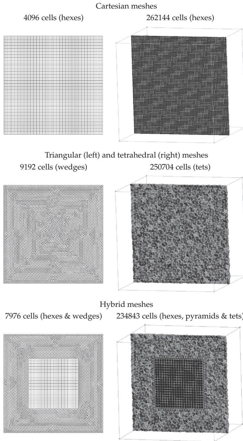
Figure 10: Meshes for the level set test cases. Left column: 2D cases; right column: 3D cases.
