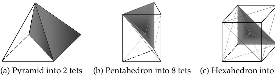
(a) Pyramid into 2 tets    (b) Pentahedron into 8 tets    (c) Hexahedron into 12 tets
