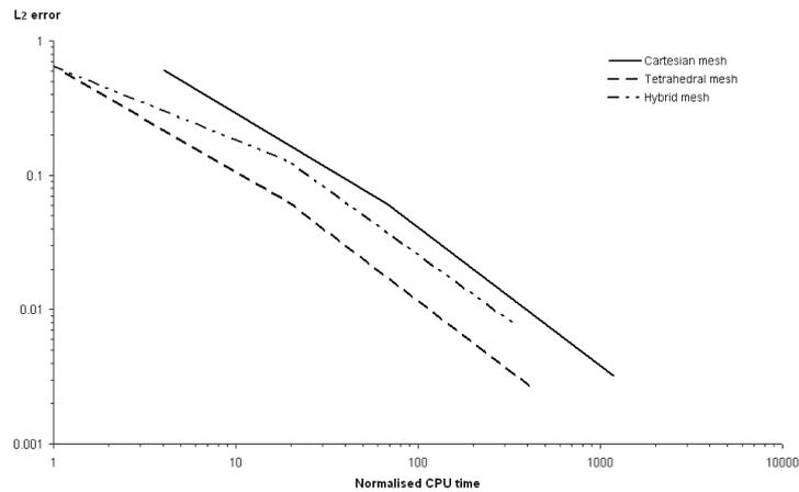
Figure 16:  $L^2$  error vs. normalised CPU time for the WENO4 applied to the linear equation.
