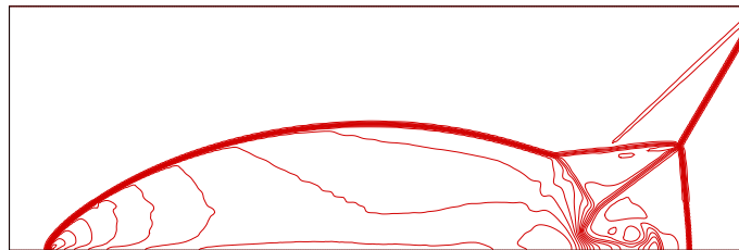
(d) 3 rd -hybrid DG/WENO-FD method (using WENO-FD flux), density 30 contours from 1.731 to 20.92, mesh size h=1/120 , t=0.2 , CPU time: 39894.4s.
