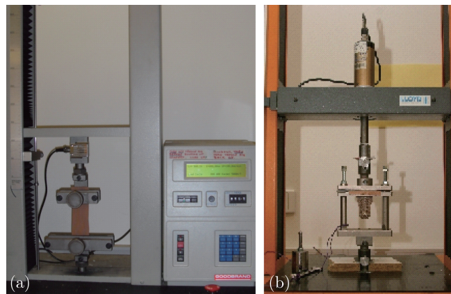
Fig. 1: Machine setup for strip fabric tensile tests (a); and fabric ball bursting strength tests (b).
