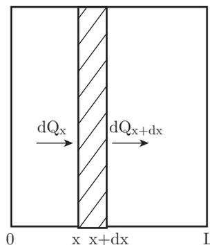
Fig. 1: Fluxional volume element of fabric heat transfer
