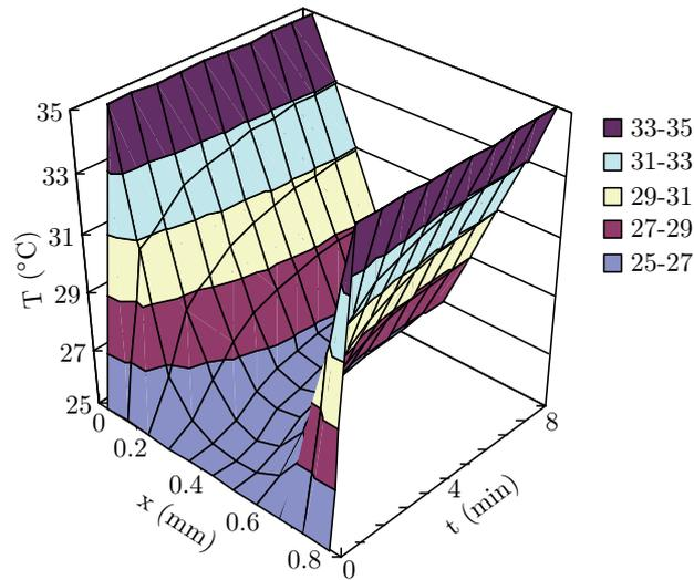
Fig. 5: Temperature distribution in the fabric
