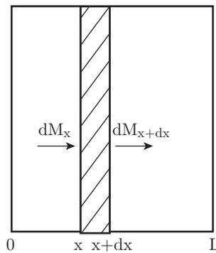
Fig. 2: Fluxional volume element of fabric mass transfer
