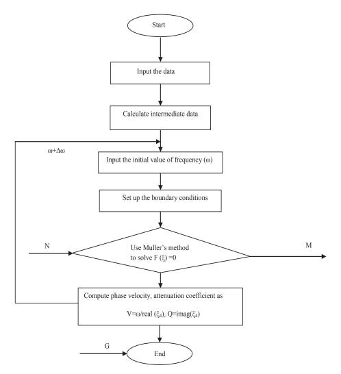
Figure 3: Flow chart for calculating phase velocity, attenuation coefficient.
