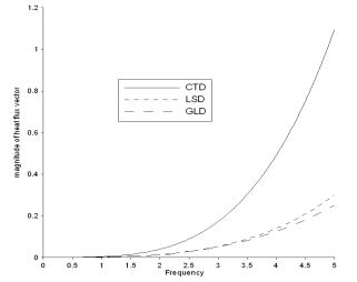
Figure 8: Variations of magnitude of heat flux vector w.r.t. frequency.
