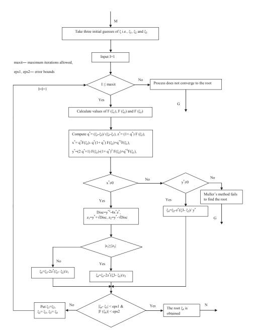
Figure 2: Flow chart to find an estimate root of  $F(\xi) = 0$ .
