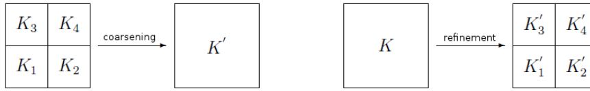
Figure 1: The sketches of coarsening (left) and refinement (right) in the adaptive mesh.
