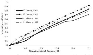
Figure 3: Comparison between non-dimensional frequency  $\Omega$  versus attunation coefficient of longitudinal modes of thermo-piezoelectric cylinderical bar immersed in fluid.
