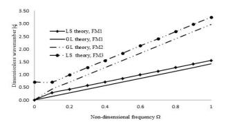
Figure 2: Comparison between non-dimensional frequency  $\Omega$  versus dimensionless wavenumber  $|\zeta|$  of Iflexural modes of thermo-piezoelectric cylinderical bar immersed in fluid.
