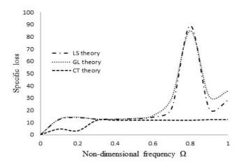
Figure 5: Non-dimensional frequency versus specific loss for longitudinal modes of thermo-piezoelectric cylindrical bar in space.
