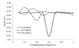
Figure 7: Non-dimensional frequency versus specific loss for longitudinal modes of thermo-piezoelectric cylindrical bar immersed in fluid.
