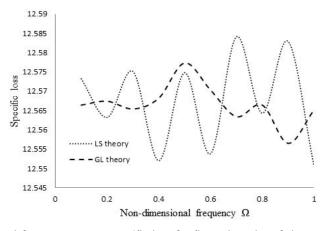
Figure 6: Non-dimensional frequency versus specific loss for flexural modes of thermo-piezoelectric cylindrical bar in space.
