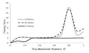
Figure 8: Non-dimensional frequency versus dimensionless daming factor for longitudinal modes of thermopiezoelectric cylinderical bar in space.
