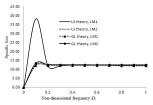
Figure 4: Comparison between non-dimensional frequency  $|\Omega|$  versus specific loss of longitudinal modes of thermo-piezoelectric cylindrical bar immersed in fluid.
