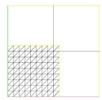
Figure 2: Triangulation and overlapping domain decomposition of  $\Omega$ .
