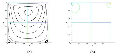
Figure 6: Computed streamlines (a) and isobars (b) for the lid-driven cavity flow at  $\nu = 0.1$ .
