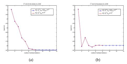
Figure 4: Evolution of the errors with the number n of nonlinear iterations at  $\nu = 0.005$ :  $|||\nabla(u - u_n^h)||_{0,\Omega} / ||\nabla u||_{0,\Omega}$  (a) and  $|||p - p_n^h)||_{0,\Omega} / ||p||_{0,\Omega}$  (b).
