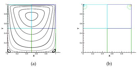
Figure 5: Computed streamlines (a) and isobars (b) for the lid-driven cavity flow at  $\nu = 1$ .
