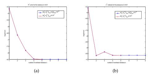
Figure 3: Evolution of the errors with the number n of nonlinear iterations at  $\nu = 0.01$ :  $|||\nabla(u - u_n^h)|||_{0,\Omega} / ||\nabla u||_{0,\Omega}$  (a) and  $|||p - p_n^h|||_{0,\Omega} / ||p||_{0,\Omega}$  (b).
