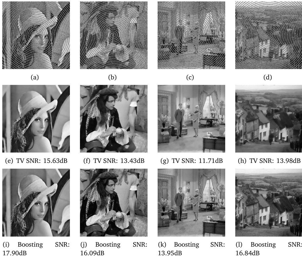
Figure 7: Gray scale image inpainting results. (a)-(d): images with missing region of level 6 and also corrupted by random Gaussian noise \sigma = 0.001 , (e)-(h): inpainted images by TV model, (i)-(l): Boosting images by our method.
