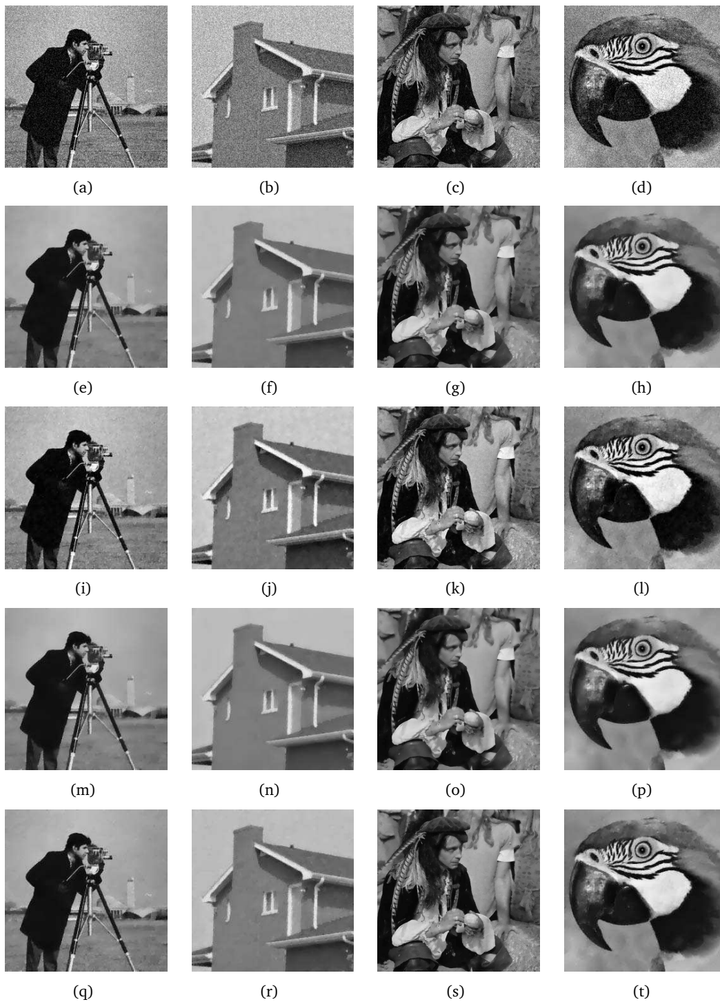
Figure 4: Gray scale image denoising results. (a)-(d): noisy images corrupted by random Gaussian noise \sigma = 20 , (e)-(h): denoised images by TV model, (i)-(l): TV boosting images, (m)-(p): TGV denoised images, (q)-(t): TGV boosting images.
