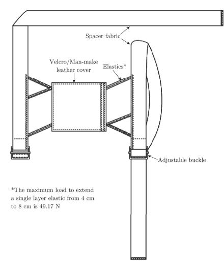
Fig. 1: Schematic diagram of a clavicle support as sourced from a local registered physiotherapist
