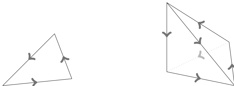
Figure 3: The Nédélec functions in \mathbb{R}^2 and \mathbb{R}^3 of the form v(x_1, x_2) = (a_1 - b x_2, a_2 + b x_1) and v(x) = a + b \wedge x , respectively, have three resp. six degrees of freedom. For each edge, the tangential component can be chosen - the resulting functions are H(\text{curl}) -conforming.
