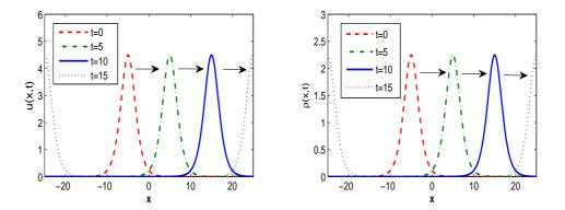
Fig. 4.1. Profile of the solitons during computing with  $\tau = 0.01$  and h = 1/8: the left one is for u(x, t) and the right one is for  $\rho(x, t)$ .
