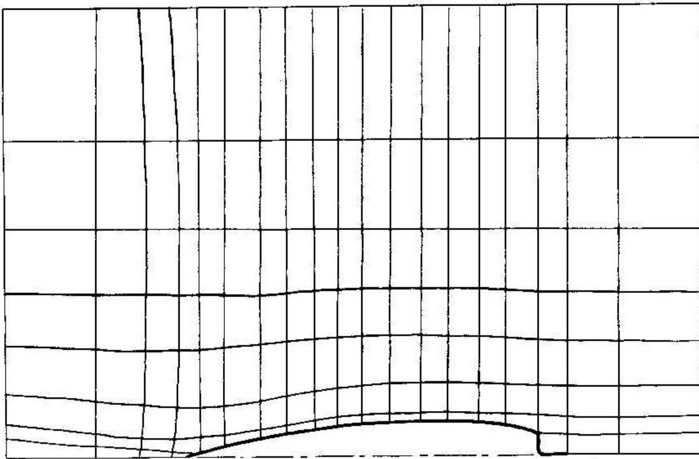
Figure 1a. Computational Grid (Longitudinal Cross Section).
