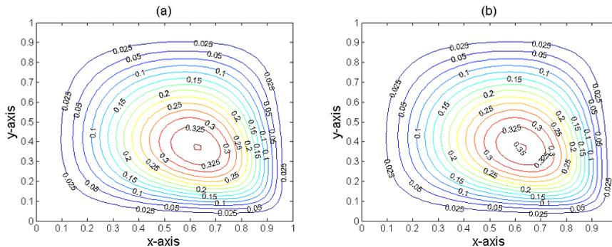
Figure 4: The deflection contour plots of the CCCC plate with exponential loading by (a) nonsingular and (b) singular BPM formulations.
