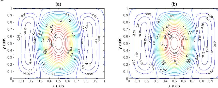
Figure 5: The deflection contour plots of the CCCC plate with trigonometric loading by (a) nonsingular and (b) singular BPM formulations.
