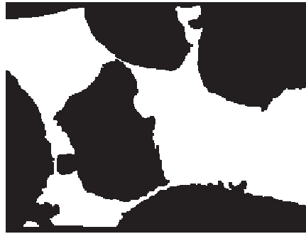
Figure 2: Illustration of a rock thin section used in the flow and solute transport simulations. Black regions refer to solid grains.
