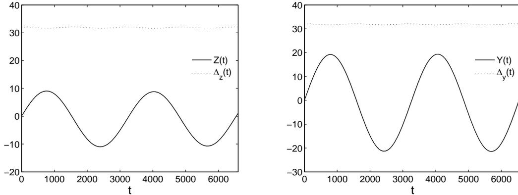
Figure 3:  $Z(t)$ ,  $Y(t)$ ,  $\Delta_z(t)$  and  $\Delta_y(t)$  for the harmonic oscillator with parameters  $N_z = N_y = 512$ ,  $\omega_0 = 2/32^2$ ,  $\tilde{m} = 1/4$ ,  $v_z = 0.02$  and  $v_y = 0.04$ . The solid lines are  $Z(t)$  and  $Y(t)$ , while the dotted ones are  $\Delta_z(t)$  and  $\Delta_y(t)$ . Time and space are expressed in lattice units.
