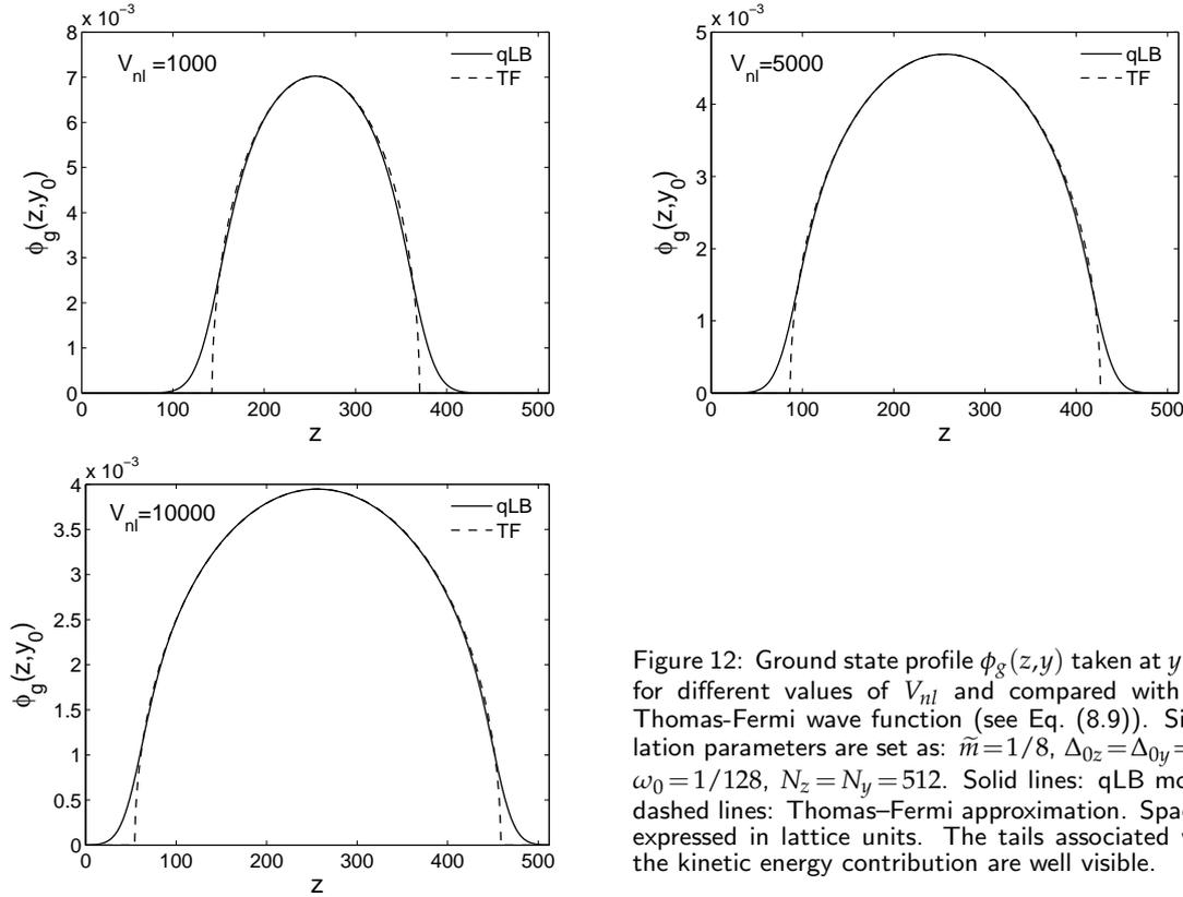
Figure 12: Ground state profile  $\phi_g(z, y)$  taken at  $y=y_0$  for different values of  $V_{nl}$  and compared with the Thomas-Fermi wave function (see Eq. (8.9)). Simulation parameters are set as:  $\tilde{m}=1/8$ ,  $\Delta_{0z}=\Delta_{0y}=16$ ,  $\omega_0=1/128$ ,  $N_z=N_y=512$ . Solid lines: qLB model; dashed lines: Thomas-Fermi approximation. Space is expressed in lattice units. The tails associated with the kinetic energy contribution are well visible.
