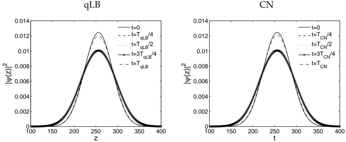
Figure 5: Wave function densities computed by qLB and CN. Parameters are set as follows:  $N_z=512$ ,  $z_0=256$ ,  $\tilde{m}=1/4$ ,  $\Delta_0=32$ ,  $\omega_0=1/512$ ,  $v_z=0.0$ ,  $V_{nl}=0.1$ . For qLB  $|\psi(z,t)|^2$  is computed at times  $0$ ,  $T_{qLB}/4$ ,  $T_{qLB}/2$ ,  $3T_{qLB}/4$  and  $T_{qLB}$ , while for CN  $|\psi(z,t)|^2$  is computed at times  $0$ ,  $T_{CN}/4$ ,  $T_{CN}/2$ ,  $3T_{CN}/4$  and  $T_{CN}$ .
