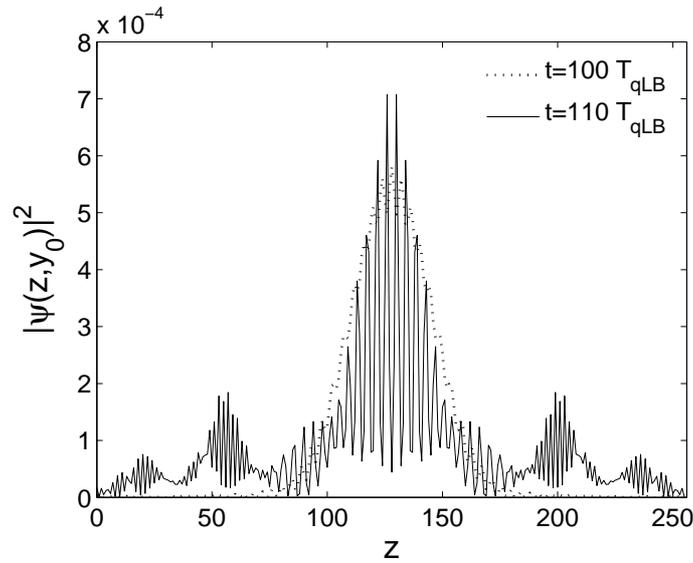
Figure 9: Wave function density computed by qLB when the BEC becomes unstable ( $V_{nl} > V_c$ ). Parameters are set as follows:  $N_z N_y = 256$ ,  $z_0 = y_0 = 128$ ,  $\tilde{m} = 1/2$ ,  $\Delta_0 = 16$ ,  $\omega_0 = 1/256$ ,  $v_z = v_y = 0.0$ ,  $V_{nl} = 2\pi$ . The wave function density is reported at times  $100T_{qLB}$  and  $110T_{qLB}$ .
