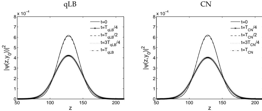
Figure 8: Wave function densities computed by qLB and CN at the cross section  $y=y_0$ . Parameters are set as follows:  $N_z=N_y=256$ ,  $z_0=y_0=128$ ,  $\tilde{m}=1/2$ ,  $\Delta_0=16$ ,  $\omega_0=1/256$ ,  $v_z=v_y=0.0$ ,  $V_{nl}=2\pi$ . For qLB  $|\psi(z,y,t)|^2$  is computed at times  $0$ ,  $T_{qLB}/4$ ,  $T_{qLB}/2$ ,  $3T_{qLB}/4$  and  $T_{qLB}$ , while for CN  $|\psi(z,y,t)|^2$  is computed at times  $0$ ,  $T_{CN}/4$ ,  $T_{CN}/2$ ,  $3T_{CN}/4$  and  $T_{CN}$ .
