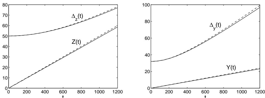
Figure 2: Comparison between  $Z(t)$ ,  $Y(t)$ ,  $\Delta_z(t)$  and  $\Delta_y(t)$  and the expected curves given by Eqs. (8.3) and (8.4) for the following setting:  $N_z = N_y = 1024$ ,  $v_z = 0.05$ ,  $v_y = 0.02$ ,  $\Delta_{0z} = 50$ ,  $\Delta_{0y} = 32$  and  $\tilde{m} = 0.2$ . Solid lines represent numerical results; dashed lines are the expected curves. Time and space are expressed in lattice units.
