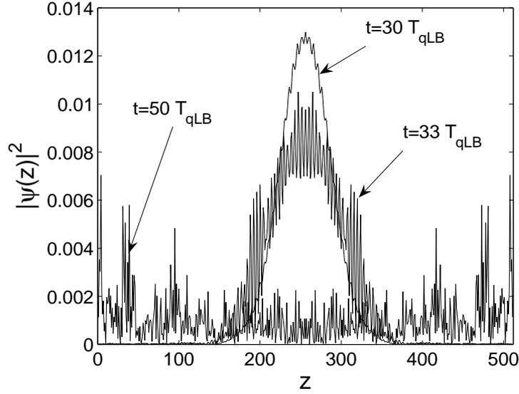
Figure 7: Wave function density computed by qLB when the BEC becomes unstable ( $V_{nl} > V_c$ ). Parameters are set as follows:  $N_z = 512$ ,  $z_0 = 256$ ,  $\tilde{m} = 1/4$ ,  $\Delta_0 = 32$ ,  $\omega_0 = 1/512$ ,  $v_z = 0.0$ ,  $V_{nl} = 0.21$ . The wave function density is reported at times  $30T_{qLB}$ ,  $32T_{qLB}$  and  $50T_{qLB}$ .
