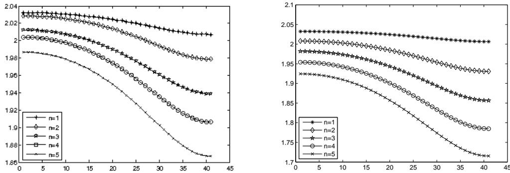
Figure 5: The values  $u_1^{(n)}$  on the interface boundary for  $n = 1, \dots, 5$  (Left: additive DDM, right: multiplicative DDM).
