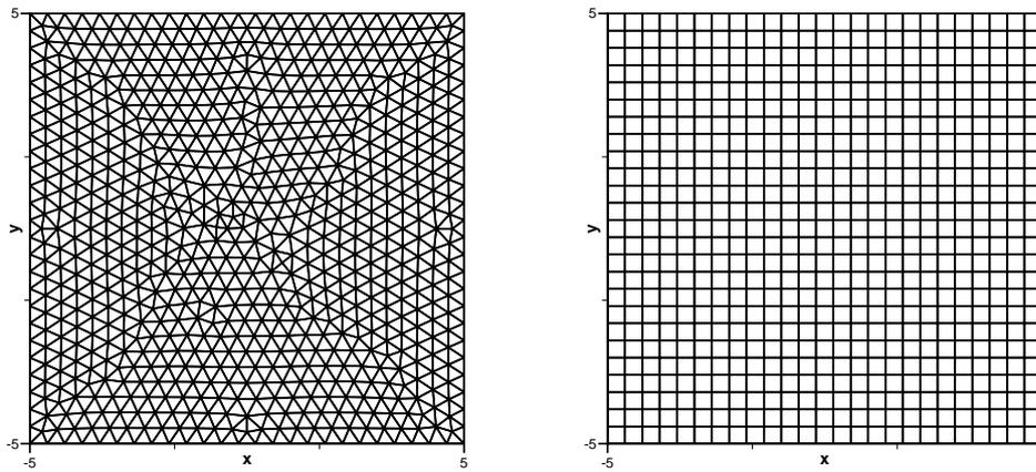
Figure 5: Uniform triangular (left) and quadrilateral (right) computational meshes used for the vortex evolution problem.
