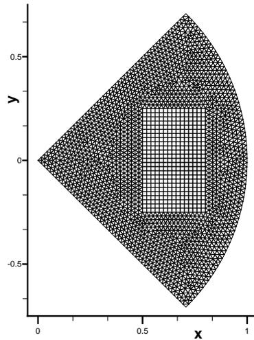
Figure 8: A mixed-element mesh with  $N_r = 50$  for the cylindrical explosion problem (5.2).
