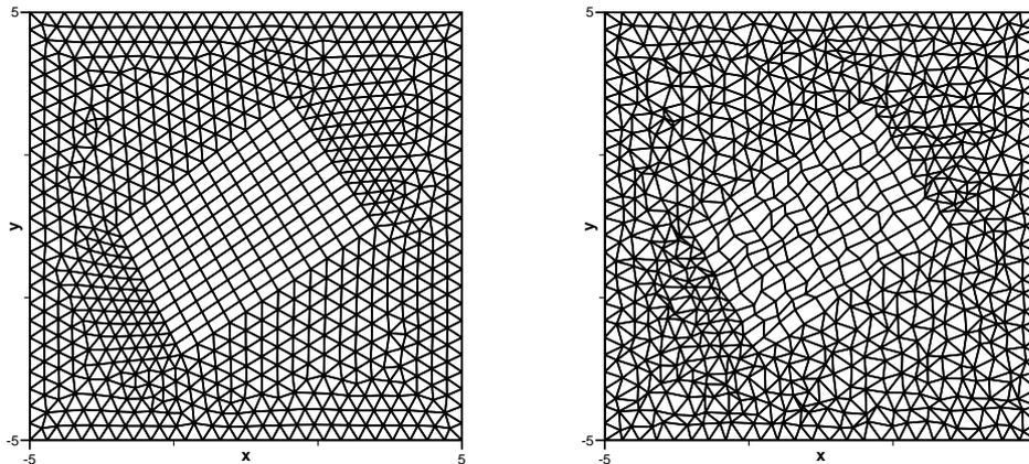
Figure 7: Uniform (left) and perturbed (right) mixed-element computational meshes with  $N=25$  used for the vortex evolution problem.
