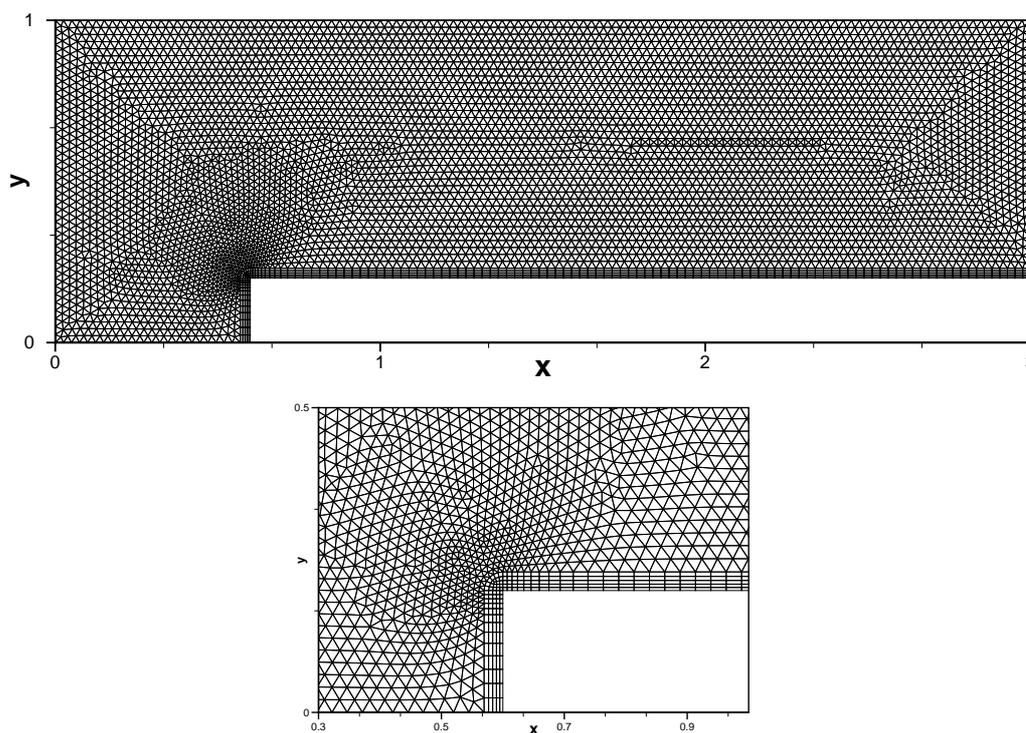
Figure 11: Mixed-element mesh for the Mach-3 wind tunnel problem.
