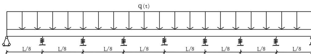
Figure 10: Flexural beam supported by nonlinear springs.
