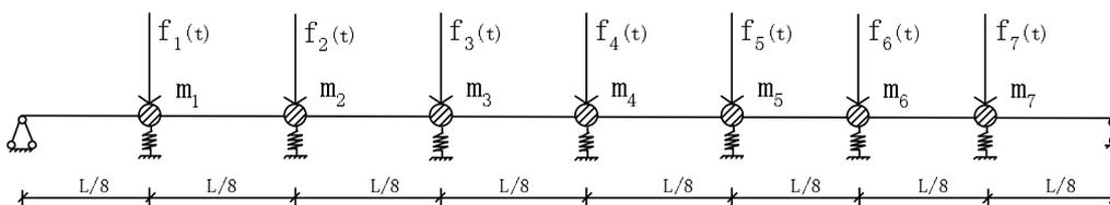
Figure 11: Model for dynamic analysis of the flexural beam.
