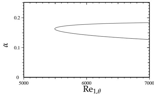
Figure 6: Neutral stability curve of two-dimensional disturbances ( $\beta=0$ ) for  $\theta=30^\circ$  for an accelerating Falkner-Skan-Cooke boundary layer with  $\alpha_{FS}=1$  and  $\beta_{FS}=0.5$ .
