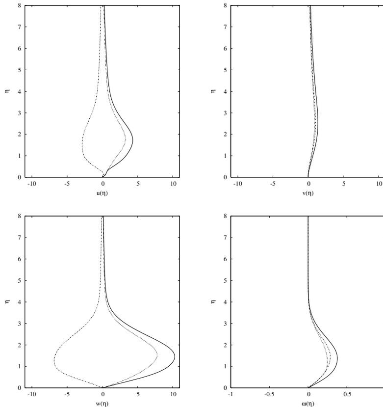
Figure 10: Eigenfunction corresponding to the most unstable eigenvalue for  $\theta = 30^\circ$  for a decelerating non-separated Falkner-Skan-Cooke boundary layer with  $\alpha_{FS} = 1$  and  $\beta_{FS} = -0.1$ ,  $Re = 346$ ,  $\alpha = 0.366$ ,  $\beta = 0.2$ . In lexicographic order:  $u$ ,  $v$ ,  $w$ ,  $\omega$ . Solid line: modulus. Dashed line: real part. Dotted-dashed line: imaginary part.
