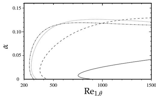
Figure 7: Neutral stability curves of three-dimensional disturbances for  $\theta=30^\circ$  for an accelerating Falkner-Skan-Cooke boundary layer with  $\alpha_{FS}=1$  and  $\beta_{FS}=0.5$ . Solid line:  $\beta=0.1$ . Dashed line:  $\beta=0.2$ . Dotted line:  $\beta=0.3$ . Dotted-dashed line:  $\beta=0.4$ .
