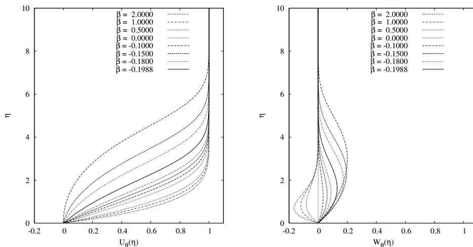
Figure 4: Velocity profiles of the Falkner-Skan-Cooke swept boundary layer for  $\theta = 45^\circ$  in a coordinate system aligned with the free stream velocity. Left: longitudinal component. Right: transverse component.
