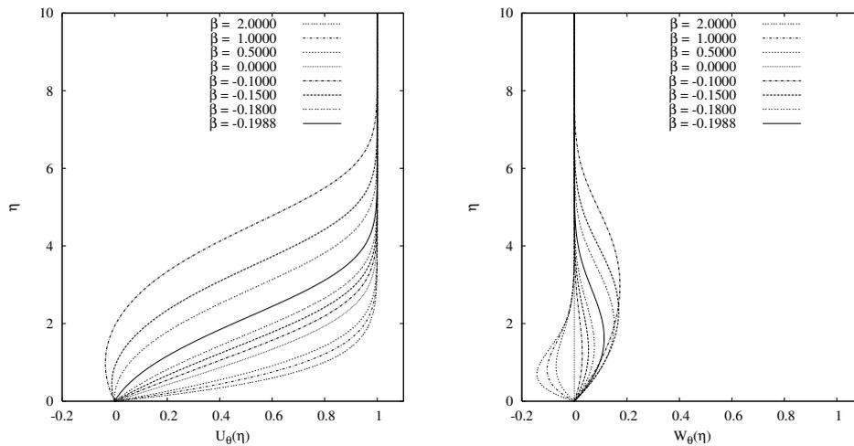
Figure 3: Velocity profiles of the Falkner-Skan-Cooke swept boundary layer for  $\theta = 30^\circ$  in a coordinate system aligned with the free stream velocity. Left: longitudinal component. Right: transverse component.
