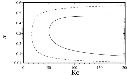
Figure 5: Neutral stability curves for two different Falkner-Skan boundary layers. Solid line: decelerating, nonseparated, boundary layer with  $\alpha_{FS} = 1$ ,  $\beta_{FS} = -0.18$ . Dashed line: decelerating, separated, boundary layer with  $\alpha_{FS} = 1$ ,  $\beta_{FS} = -0.18$ .
