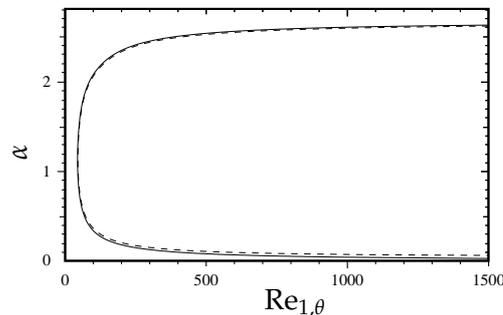
Figure 9: Neutral stability curves of two and three-dimensional disturbances for  $\theta = 30^\circ$  for a separated Falkner-Skan-Cooke boundary layer with  $\alpha_{FS} = 1$  and  $\beta_{FS} = -0.1$ . Solid line:  $\beta = 0$ . Dashed line:  $\beta = 0.1$ .
