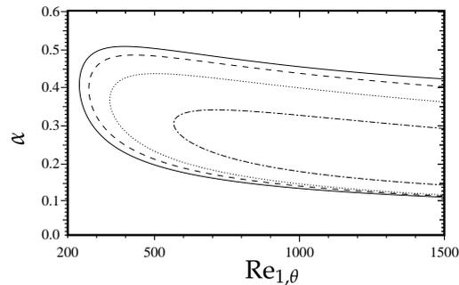
Figure 8: Neutral stability curves of two and three-dimensional disturbances for  $\theta = 30^\circ$  for a decelerating Falkner-Skan-Cooke boundary layer with  $\alpha_{FS} = 1$  and  $\beta_{FS} = -0.1$ . Solid line:  $\beta = 0$ . Dashed line:  $\beta = 0.1$ . Dotted line:  $\beta = 0.2$ . Dotted-dashed line:  $\beta = 0.3$ .
