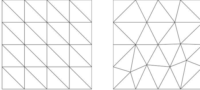
Figure 2: Structured (left) and unstructured (right) triangulations of the computational domain.
