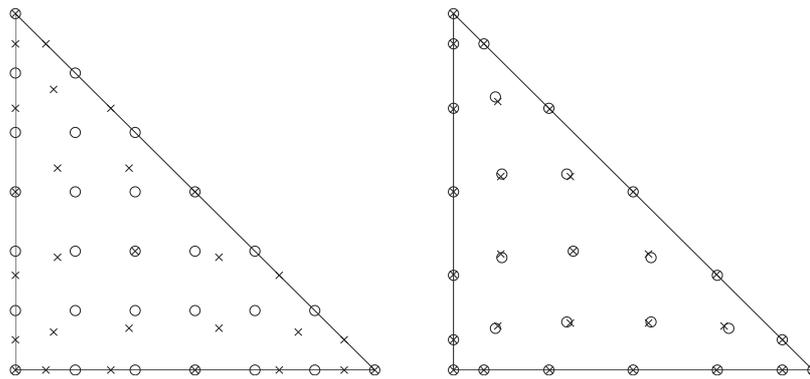
Figure 3: Different collocation points for  $p=6$ . Left: Uniform ( $\circ$ ) and Fekete ( $\times$ ) points. Right: Lobatto ( $\circ$ ) and Lebesgue ( $\times$ ) points.
