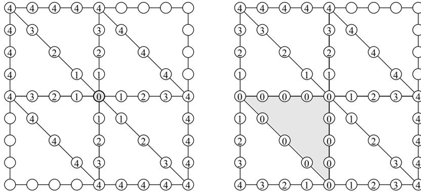
Figure 1: Distance function of a node from a vertex (left) and from an element (right) in the case  $p=4$ . The distance is infinity for nodes without a number.
