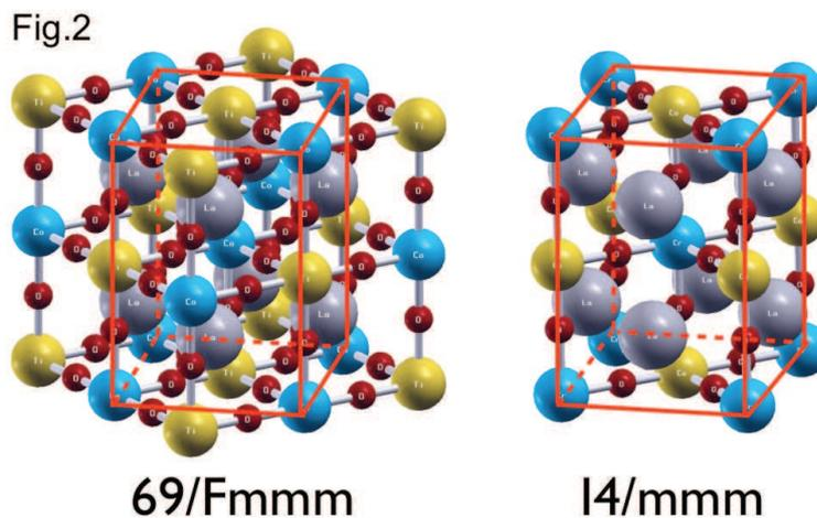
Figure 2: Double perovskite structure in space group  $69/Fmmm$  and  $I4/mmm$ .
