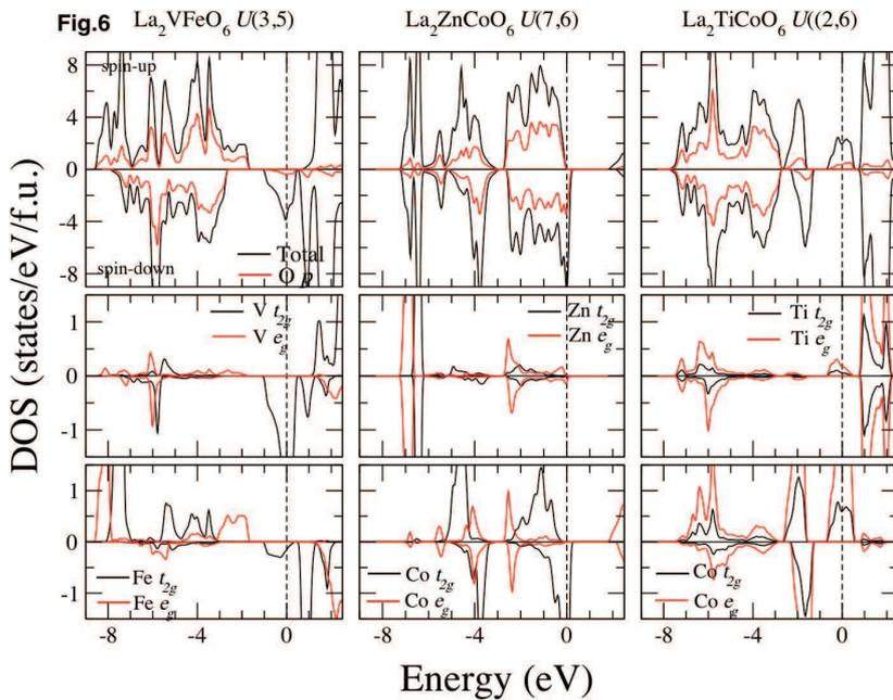
Figure 6: Calculated total, spin, and site-decomposed density of states of  $\text{La}_2\text{VFeO}_6$ ,  $\text{La}_2\text{ZnCoO}_6$ , and  $\text{La}_2\text{TiCoO}_6$  in GGA+ $U$  process.
