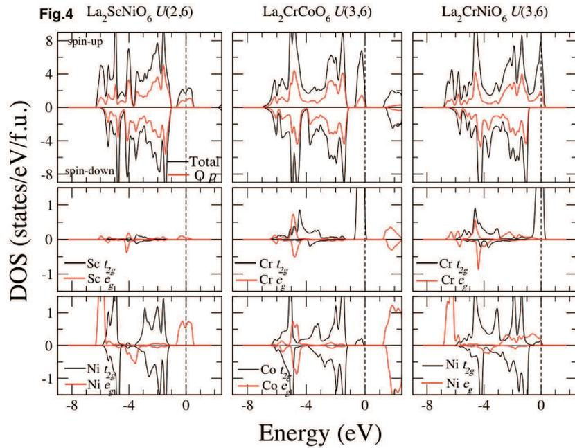
Figure 4: Calculated total, spin, and site-decomposed density of states of  $\text{La}_2\text{ScNiO}_6$ ,  $\text{La}_2\text{CrCoO}_6$ , and  $\text{La}_2\text{CrNiO}_6$  in GGA+U process.
