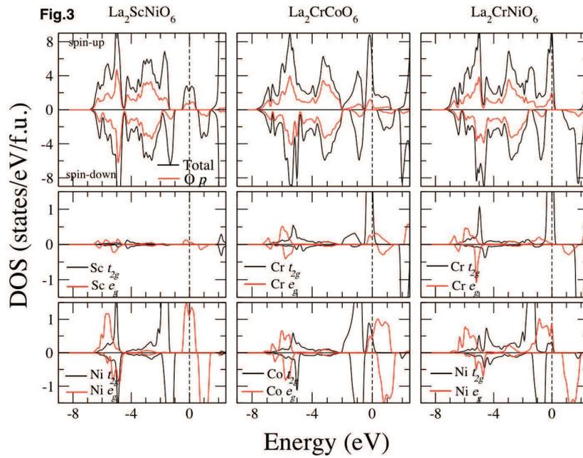
Figure 3: Calculated total, spin, and site-decomposed density of states of  $\text{La}_2\text{ScNiO}_6$ ,  $\text{La}_2\text{CrCoO}_6$ , and  $\text{La}_2\text{CrNiO}_6$  in GGA process.
