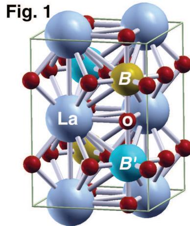
Figure 1: An ideal ordered double perovskite structure  $\text{La}_2\text{BB}'\text{O}_6$ . For FiM state, the spin state of  $(B, B, B', B')$  is  $(+, +, -, -)$ . For AF state, the spin state of  $(B, B, B', B')$  is  $(+, -, +, -)$ .
