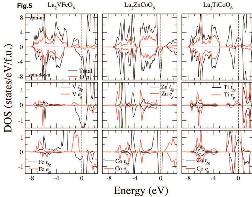
Figure 5: Calculated total, spin, and site-decomposed density of states of  $\text{La}_2\text{VFeO}_6$ ,  $\text{La}_2\text{ZnCoO}_6$ , and  $\text{La}_2\text{TiCoO}_6$  in GGA process.
