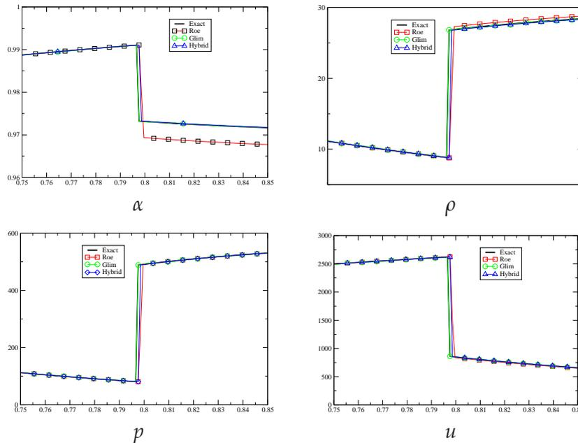
Figure 6: Zoom of the physical variable around the shock location.
