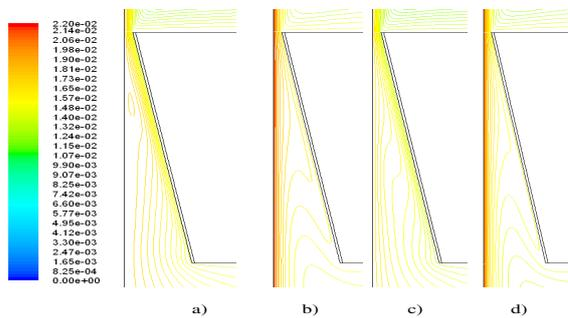
Figure 7: Air streamlines ( $\text{kg}/\text{sm}^2$ ), for  $q_w = 120\text{W}/\text{m}^2$ ,  $b = 20\text{mm}$  and  $\theta = 10^\circ$ : (a)  $V_b = 0\text{m}/\text{s}$ ,  $\epsilon_p = \epsilon_b = 0$ ; (b)  $V_b = 1\text{m}/\text{s}$ ,  $\epsilon_p = \epsilon_b = 0$ ; (c)  $V_b = 0\text{m}/\text{s}$ ,  $\epsilon_p = 0.90$ ,  $\epsilon_b = 0.20$ ; (d)  $V_b = 1\text{m}/\text{s}$ ,  $\epsilon_p = 0.90$ ,  $\epsilon_b = 0.20$ .
