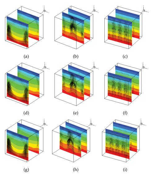
Figure 4: Velocity vectors and temperature on two cross-sections for different magnetic Rayleigh numbers: (a)-(c) Ram = 0, (d)-(f)  $Ram = 1.0 \times 10^7$ , (g)-(i)  $Ram = 1.25 \times 10^7$ .
