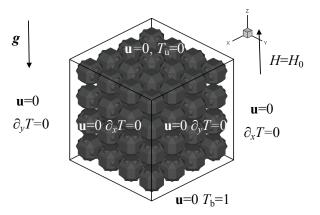
Figure 2: Porous media simulation boundary conditions.
