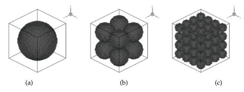
Figure 1: Porous media simulation cells: (a) 1 ball, (b) 8 balls, (c) 64 balls.
