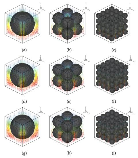
Figure 3: Velocity vectors for different magnetic Rayleigh numbers: (a)-(c) Ram = 0, (d)-(f)  $Ram = 1.0 \times 10^7$ , (g)-(i)  $Ram = 1.25 \times 10^7$ .
