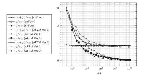
Fig. 4.4. Efficiency indices for uniform mesh-refinement, adaptive mesh-refinement (Variant 1) and adaptive mesh-refinement (Variant 2) with  $e_H := ||D_{NC}^2(u - u_H)||$ .
