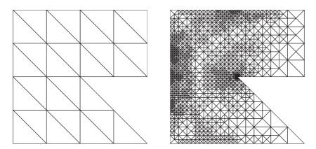
Fig. 4.2. Left: initial mesh. Right: adaptive mesh generated by AFEM Variant 2 in level 10 of the adaptive loop; the number of triangles is 2730.
