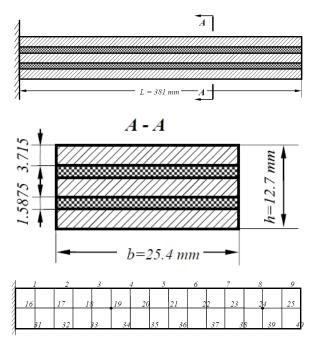
Figure 4: A multilayer sandwiched beam structure with viscoelastic damping.
