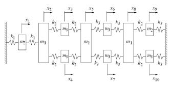
Figure 2: A mass-spring vibration model used as numerical example with  $m_1 = 1.0$ kg,  $m_2 = 0.2$ kg,  $m_3 = 0.1$ kg,  $k_1 = 1.0 \times 10^6$ N/m,  $k_2 = 2.0 \times 10^6$ N/m.
