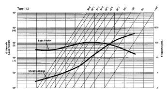
Figure 1: Reduced frequency nomogram for ISD-112.
