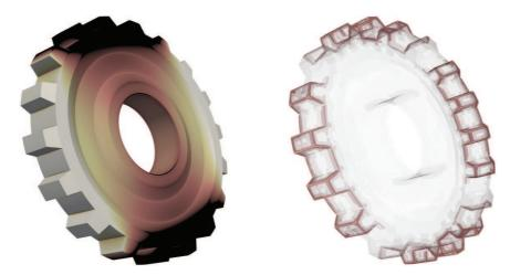
Fig. 5.3. Solution (left) and refinement (right) on the gearwheel with a smooth right-hand side.
