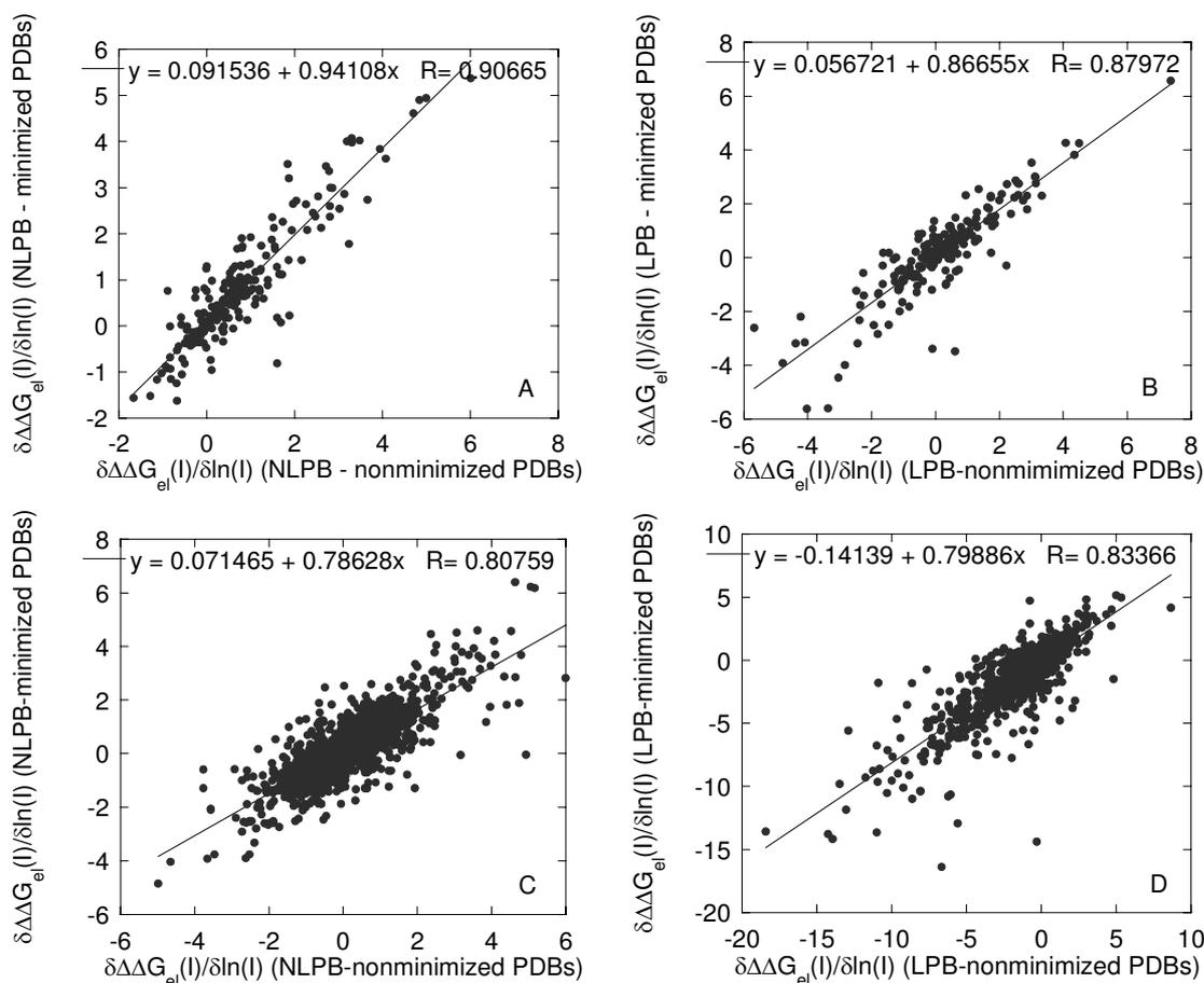
Figure 3: Fitting slopes ( $\delta\Delta\Delta G_{el}(I)/\delta\ln(I)$ ) calculated with (A,C) NLPB and (B,D) LPB compared for non minimized and minimized structures for hetero- and homo-complexes, respectively.
